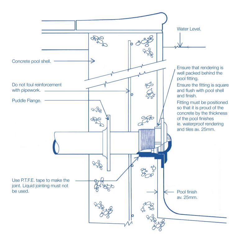
**Important:** All pipework and pool fittings must be pressure tested before backfilling and commissioning. Drawing is not to scale.
