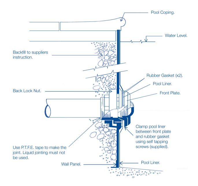
**Important:** All pipework and pool fittings must be pressure tested before backfilling and commissioning. Drawing is not to scale.
